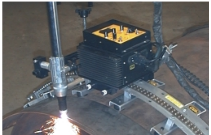
Hi-Flex Rail (FMD) for various circumferential and irregular surface applications down to 30" (760 mm) radius. (Page 5)
